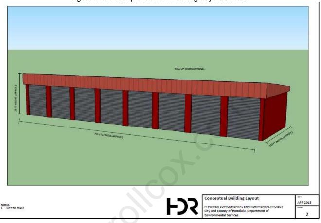
Figure S2: Conceptual Solar Building Layout Profile
