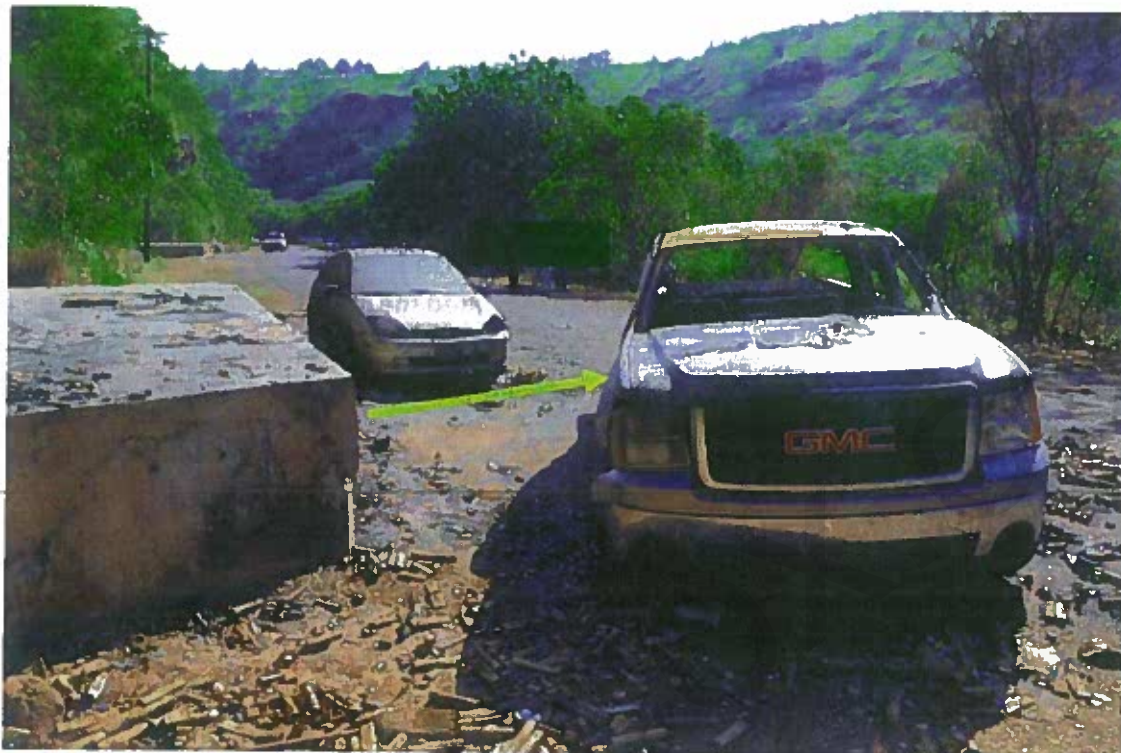
Figure 21. Prior to incident, this GMC truck was parked just in front of the silver car. The force of the explosion moved the rear of the truck to the right as indicated by the arrow.
