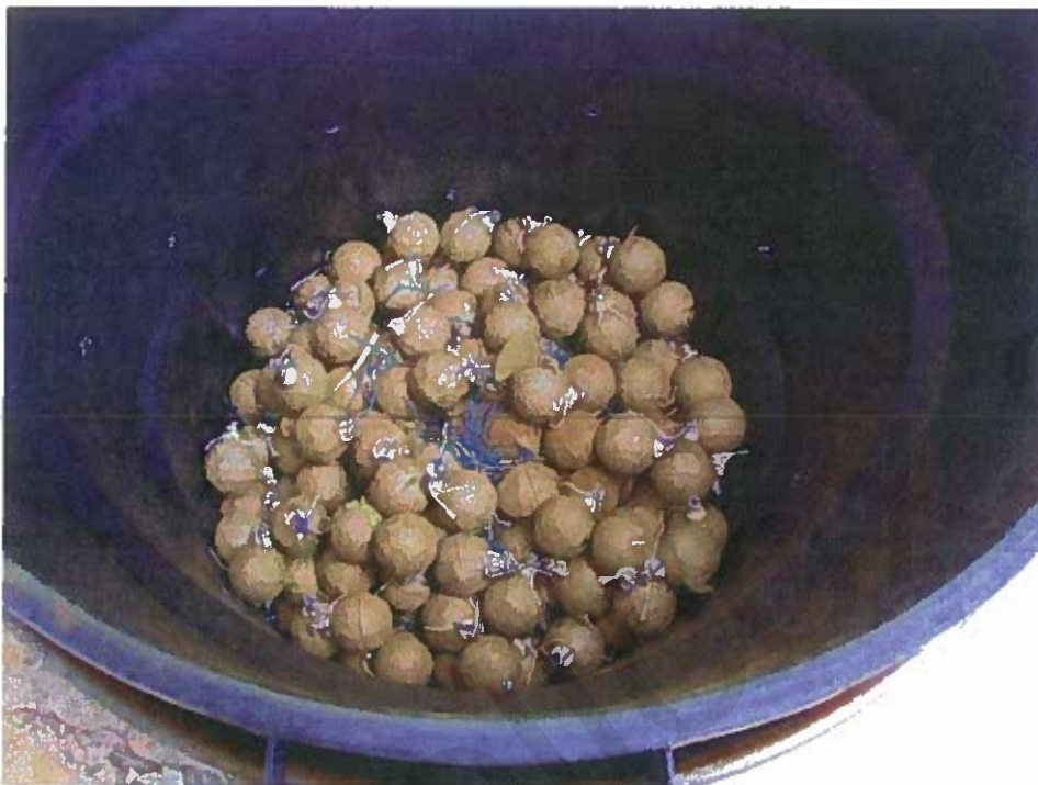
Figure 9. Aerial shells removed from the firework tubes and placed in an inner liner for diesel soaking
