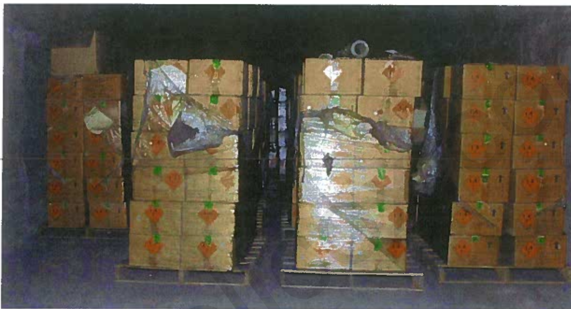
Figure 18. 2009 Seizure (second seizure) at rear of magazine, relatively undamaged with some melting of the plastic wrapping following the explosion and fire near the front of the magazine.
