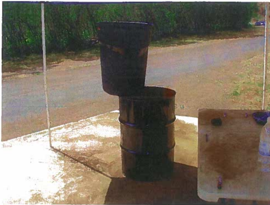
Figure 8. 55 gallon steel drum and inner liner used for diesel soaking
